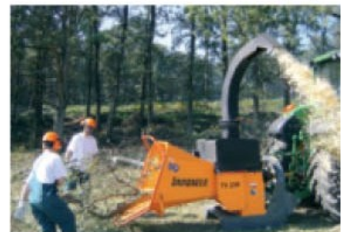
TV250 P; The large infeed opening, combined with an aggressive infeed system guarantees high productivity.
