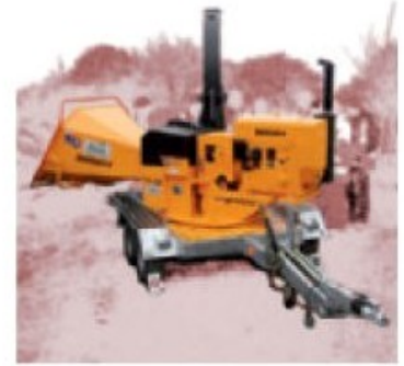
TV180 D ; Comes standard on a road trailer with tandem axle, 360° turning.
