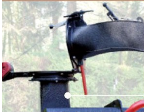
Foldable ejector chute with manual winch (optional)
