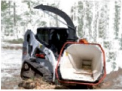
Hydraulic driven version for tool carriers.
