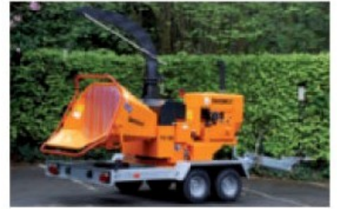
Diesel engine driven version with road trailer
