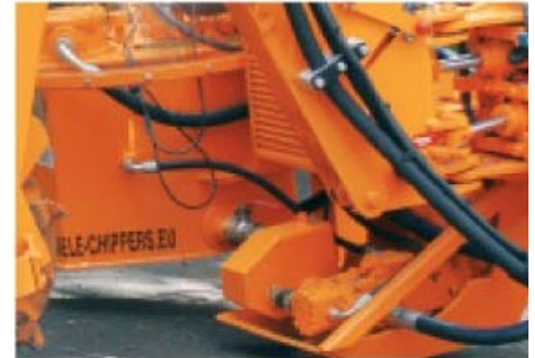
Integrated hydraulic group: pumps, oil tank and oil cooler:
